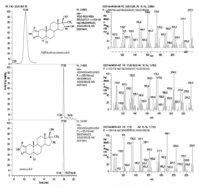
Fig. 3. LC-MS chromatogram and spectrum of 16-OHStan, Stanozolol-d<sub>3</sub>, Stan.
